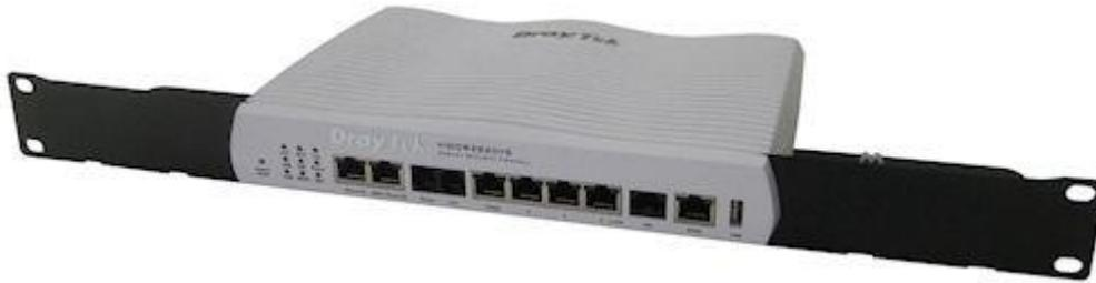
The RM1 Rackmount Bracket enables you to fit any Vigor2860 series router into a standard 19" rack or cabinet. The bracket takes up one rack slot (1U) and includes a cable retainer at the back to keep the power cord captive. The front mounted sockets of the router remain fully accessible. For wireless models, we then recommend extension aerials (or aerial extensions).
